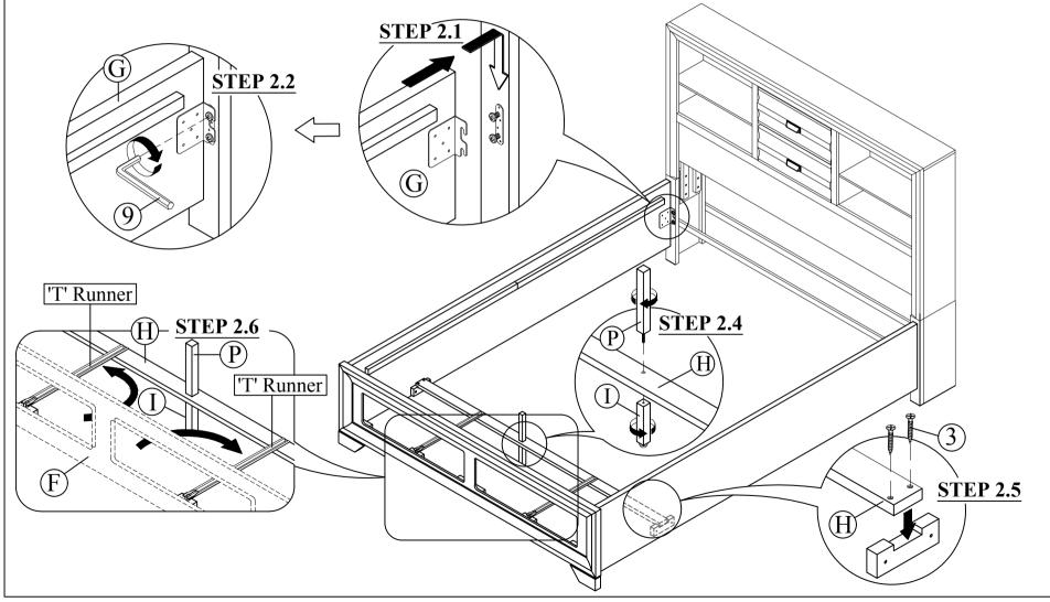
NOTE: MUST TIGHTEN SCREWS PERIODCALLY WITH USE SCREW WILL BECOME LOOSE. CHECK TIGHTNESS OF ALL SCREW EVERY 6-8 WEEKS.
