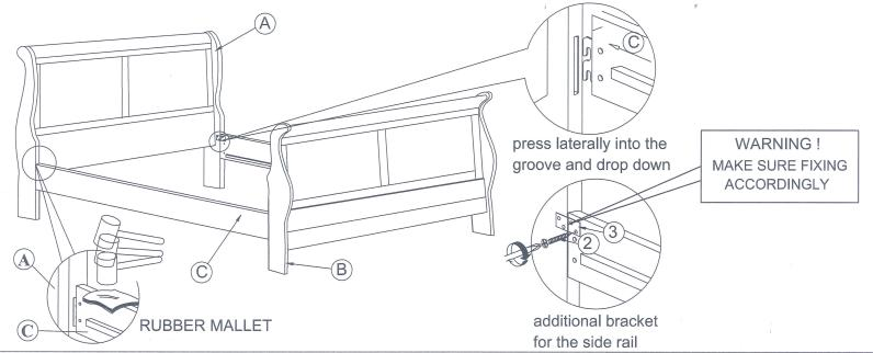
STEP 2 : Attach the Bed slat support (E) with adjuster to Side Rail (C) as picture shown. Loosen and tighten Adjuster for the stability of bed. Lastly, tighten the Bed slat (D) with CSK Screw (1).
